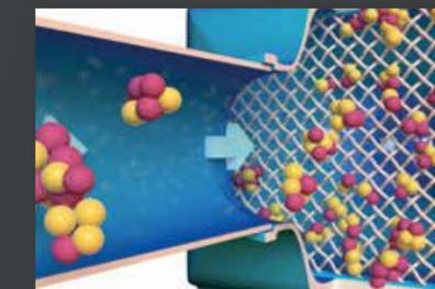
The suspended crystals of hard water elements are retained in the filter cartridge leaving soft water in the spa.
