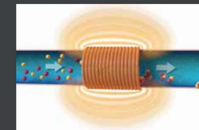
The system generates an electro-magnetic field that agitates calcium and other minerals in the water, causing them to create suspended crystals.
